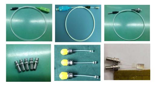
W2 also developed unique receptacle with isolator integrated with tapped lens for TOSA applications.
